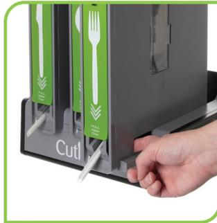
If it's still not ready for dispensing, the cutlery pack may be jammed. Pull the cartridge out and push the small latch on the front, middle underside to open the bottom; remove all cutlery and reload.
